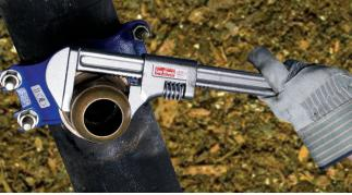
Major brass fittings manufacturers recommend RCORP when tightening corp stops, either into the pipe or tapping saddle, or tightening service line connections on any waterworks brass valve or fitting.
